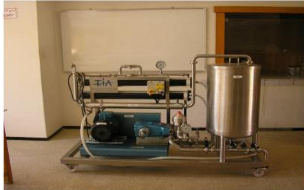
Schematic diagram and picture of the nanofiltration/reverse osmosis pilot plant. T: tank; P: feed pump; V: pressure regulation valves; M: nanofiltration module; Pe: permeate recirculation; R: retentate recirculation; H: heat exchanger; 1: pressure sensor; 2: temperature sensor.
